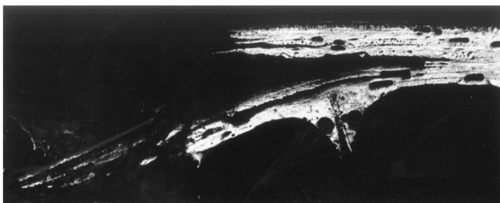
Figure 4 Photomicrograph of a Nomex core bay impacted with 8.1 J at 25 \times magnification.
